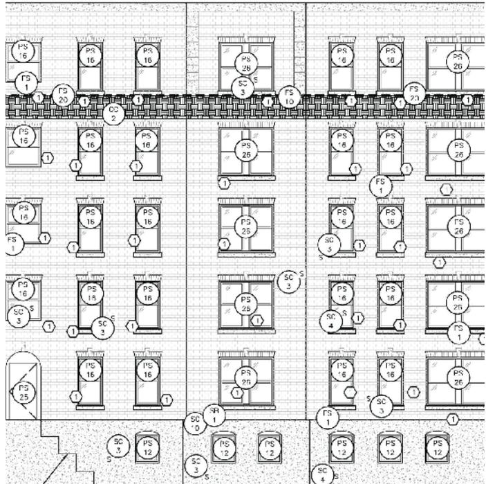
*Elevations drawings can be annotated to indicate the location(s) and scope(s) of work to be performed.*
