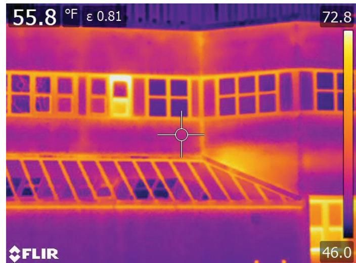
*Infrared Thermography shows temperature differences, which can indicate moisture, air leakage, and thermal bridges within the building enclosure.*
