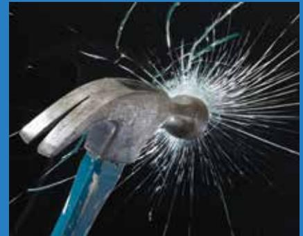
Figure 1: Laminated glass has both safety and security uses, and also enhances sound attenuation and ultraviolet protection.
